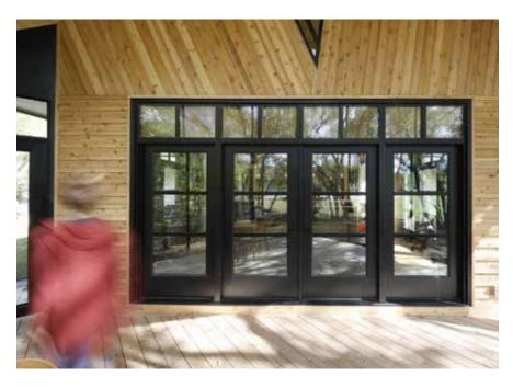
**ABOVE** Series 458 Inswing French Doors with Astragal in Black, Series 458 Fixed Doors (Sidelites), Flush Glazed 42x84" Panels, Triple Pane LoE 272/180 Argon glass with 2" Flat SDLs, Narrow Perimeter, Profiled Brickmould, and Multi-Point with Lever in Black.
