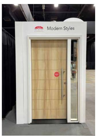
Series 658 Inswing with Fixed Sidelite in White, Grooved Wheat Stain on Cherry Grain C999 Panel, Triple Pane Low-E Argon glass, Narrow Perimeter, Flat Expander, and Multi-Point Lock with Short Pull Bar in Stainless Steel.
